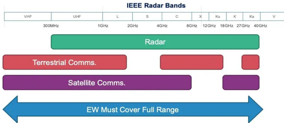
Figure 1: IEEE radar bands with common uses.
